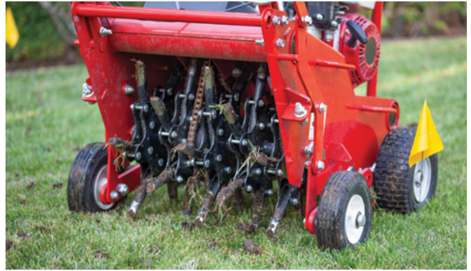
Figure 25b. Core aeration machines remove narrow plugs of compacted soil. (Adobe Stock)
