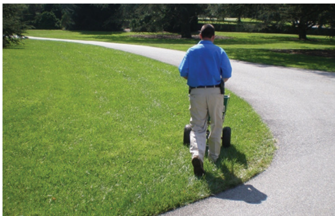
Figure 15. Some rotary spreaders are equipped with edge guards that block one side of the spread pattern, which makes it easier to apply fertilizer along the edge of a non-target area. (Peter Landschoot)
